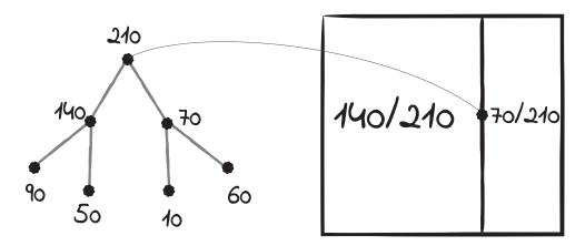
The algorithm proceeds top-down to split the area according to the size proportions of the first level of nodes.
